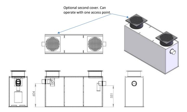
Where a Mactrap passive trap is installed underground and the access points are lower than ground level, risers can be added to any of the Mactrap range. These can either be welded to the tank, or provided separately and welded to the tank when in situ. The risers are made from the same HDPE as the tank. The Class A (Pedestrian) and Class D (Traffic) lids are sealed and are manufactured to Class A & D specifications.
