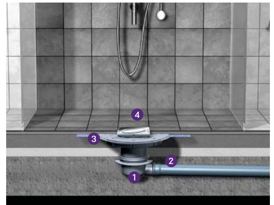
① Drain ② Outlet ③ Adhesive flange ④ Steel cover
