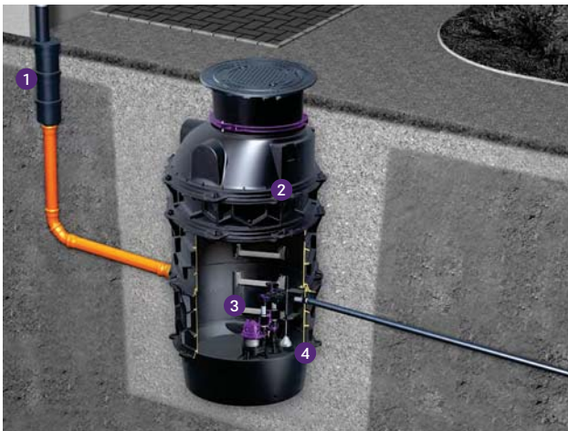
1 Gutter drain 2 Pumping station 3 Pump 4 Pressure sensor
