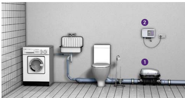
1 Backwater valve 2 Control unit
