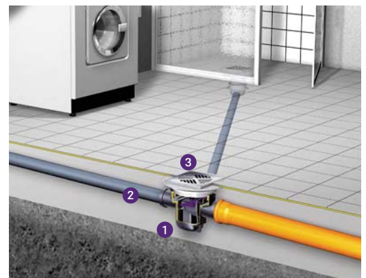
1 Drain 2 Inlet 3 Steel cover
