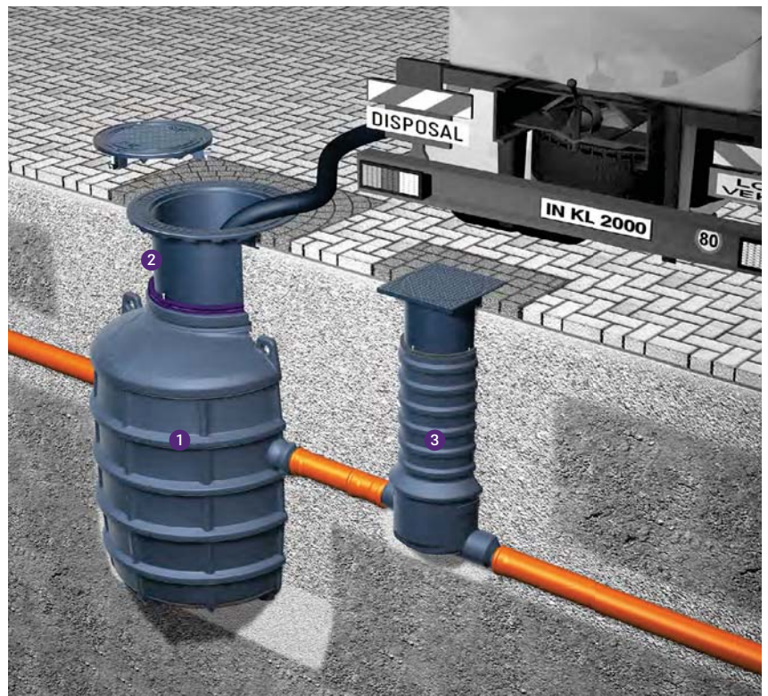
1 Grease separator 2 Height adjustable upper section 3 Sampling chamber
