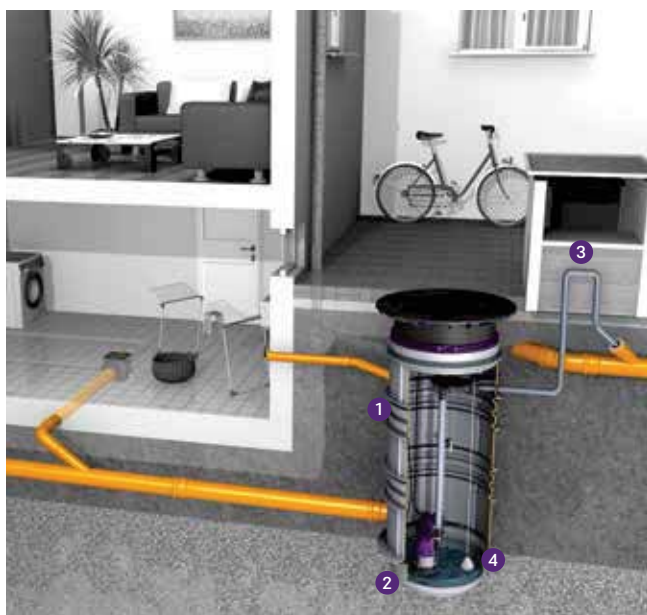
1 Pumping station 2 Pump 3 Pressure pipe 4 Pressure sensor
