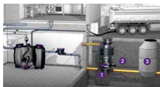
1 Hybrid lifting station 2 Pressure pipe 3 Pressure relief chamber
