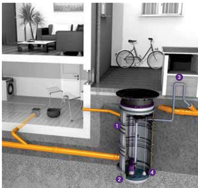
1 Pumping station 2 Pump 3 Pressure pipe 4 Pressure sensor
