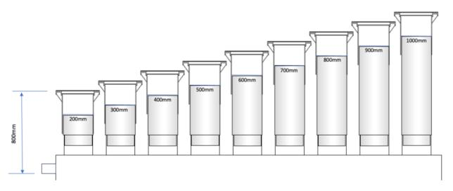
Installation depth of greater than 1 metre requires a static load bridge.
