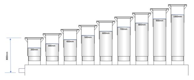
Installation depth of greater than 1 metre requires a static load bridge.
